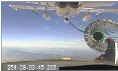
Figure 1 | The Autonomous Airborne Refueling Demonstration (AARD) program was a DARPA-funded demonstration of in-flight refueling using an autonomous aircraft. A GE COTS image processor card provided near-flawless detection, clutter rejection, and rigorous tracking of the refueling drogue in three dimensions.
