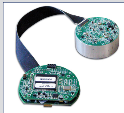
Figure 3 | Three DSP-1750 Fiber Optic Gyros from KVH are used in the company's 1750 Inertial Measurement Unit that is about the size of a coffee cup.
