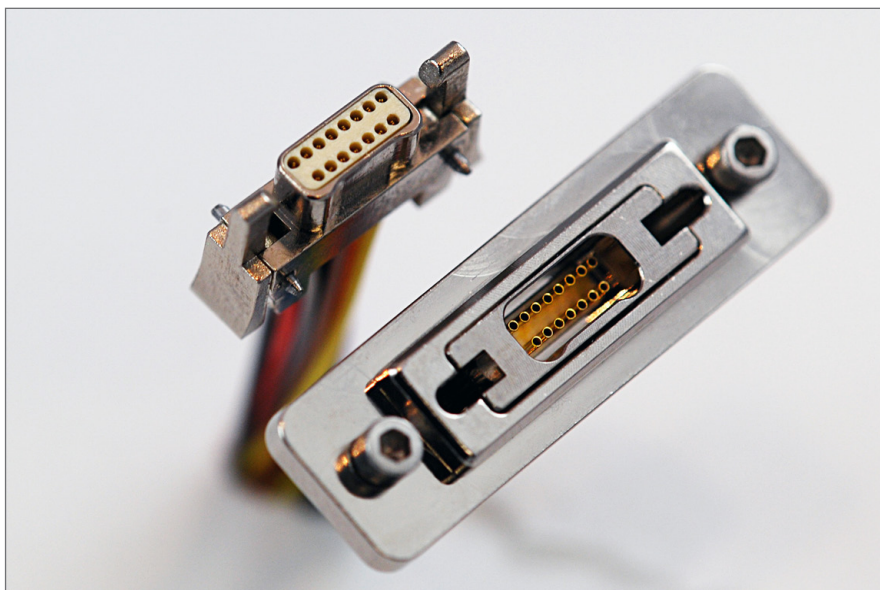
Figure 1 | BiLobe connectors can handle a shock of 100 g in each axis and have passed vibration testing from 10 to 2,000 to 10 Hz at 20 g amplitude in each axis.
